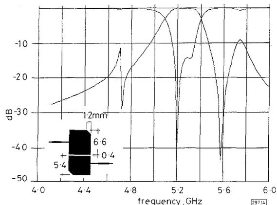
Fig. 4 Predicted performance by computer simulation of slot coupled dual-mode bandpass filter with different transversal lengths of patches
