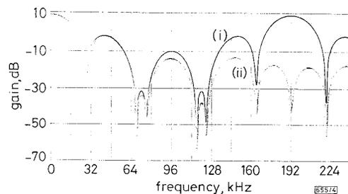
Fig. 4 Computer simulation results of SC interpolator
