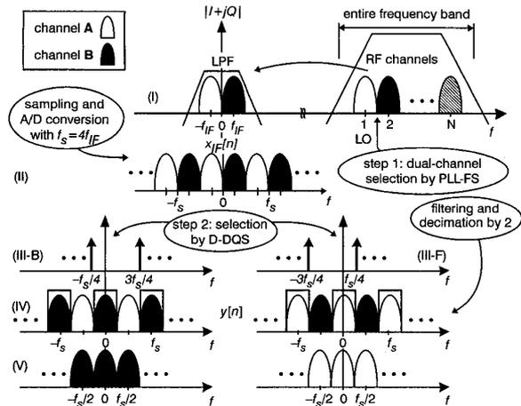
Fig. 3 Spectra flows of proposed channel selection method
