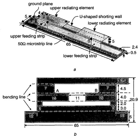
**Fig. 1** Geometry of proposed metal-plate 1 × 2 array antenna for WLAN operation in 5.2/5.8 GHz bands, and proposed antenna unfolded into planar metal plate
