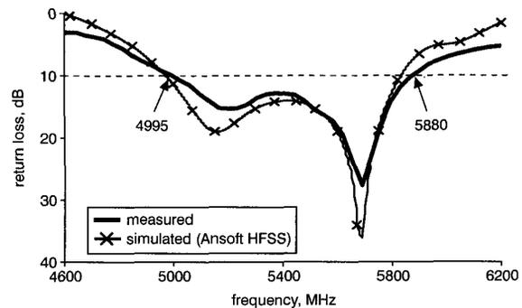
**Fig. 2** Measured and simulated return loss
