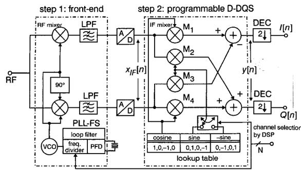
Fig. 2 New proposed complex low-IF receiver topology
