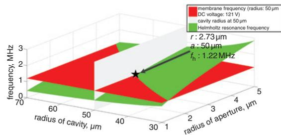
**Fig. 2** Determining dimensions of Helmholtz aperture from parameters of CMUT membrane
