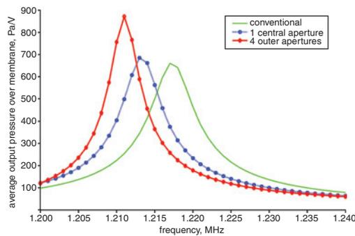
**Fig. 5** Average output pressure over membrane: comparison between CMUTs with Helmholtz resonance apertures and conventional CMUT
