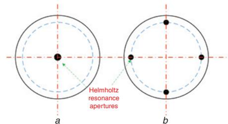
**Fig. 3** Configuration of CMUT with one (Fig. 3a) and four (Fig. 3b) Helmholtz resonance apertures (radius of apertures are: 2.73  $\mu\text{m}$  for single central aperture and 1.37  $\mu\text{m}$  for four apertures)
