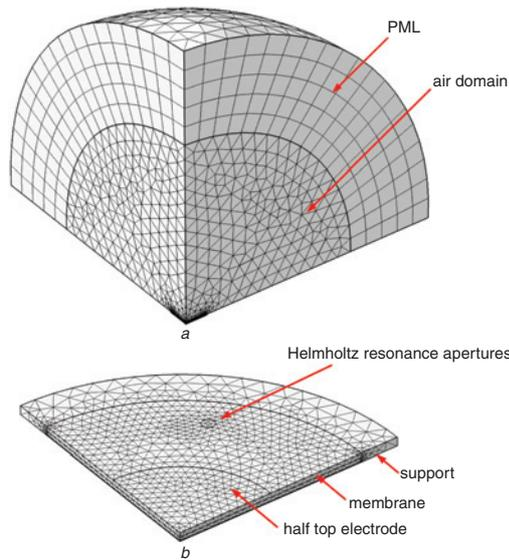
**Fig. 4** 3D FEA model of CMUT cell and air domain: CMUT cell and air domain (Fig. 4a) and details of CMUT cell (Fig. 4b)
