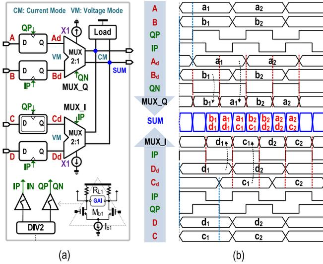
Fig. 2. (a) Implementation of the TI-DBTX and (b) its timing chart.
