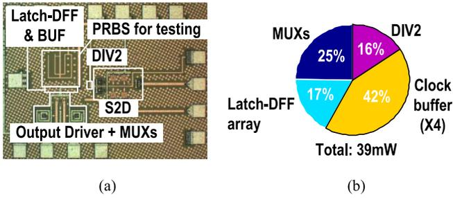
Fig. 5. (a) Die photograph and (b) power breakdown of the fabricated TI-DBTX.
