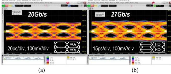
Fig. 6. Measured eye diagrams at (a) 20 and (b) 27 Gb/s.
