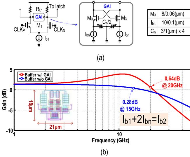
Fig. 3. (a) Swing-enhanced clock buffer using a GAI. (b) Simulated gain responses with and without GAI.
