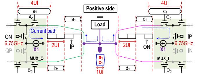
Fig. 4. Unified 4-to-2 MUX-and-SUM operation.
