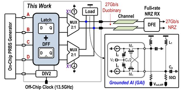
Fig. 1. System architecture of the proposed TI-DBTX.
