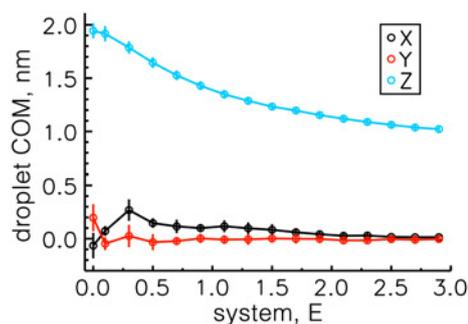
**Fig. 4** Location of the droplet on the surface: *X* and *Y* are deviations of the droplet's COM from the middle of the electrode pairs; *Z* is the distance of COM from the first layer of atoms in the hydrophobic surface. Error bars are standard deviations
