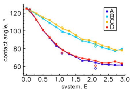
**Fig. 3** Regional contact angle (A, B, C and D, see Fig. 1) in the presence of an applied electric field. Simulation results of larger box size  $30 \times 30 \times 30$  are plotted as circle. Standard errors range from  $0.11^\circ$  to  $1.0^\circ$
