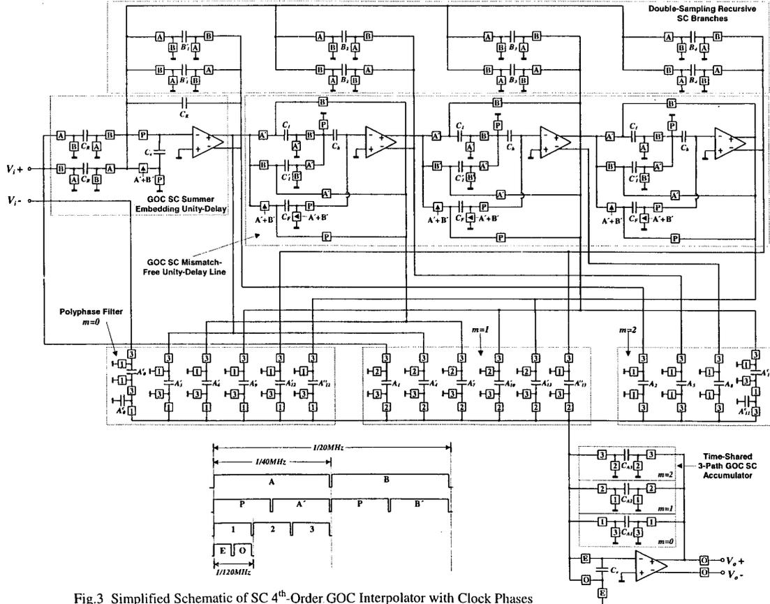
Fig.3 Simplified Schematic of SC 4<sup>th</sup>-Order GOC Interpolator with Clock Phases
