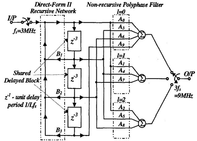
Fig.1 Recursive ADB Polyphase Structure for 3<sup>rd</sup> Order IIR Lowpass Interpolation
