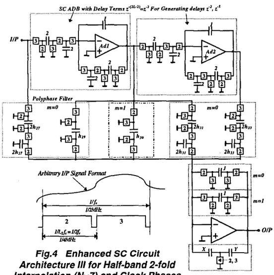
**Fig.4 Enhanced SC Circuit Architecture III for Half-band 2-fold Interpolation ( $N=7$ ) and Clock Phases**
