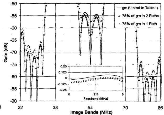
Fig. 4 OTA finite gain and bandwidth effects for 2-stage SC anti-imaging filter – Amplitude response simulations with one-pole OTA model, parasitic capacitance of OTA, SC branches and non-zero switch resistance
