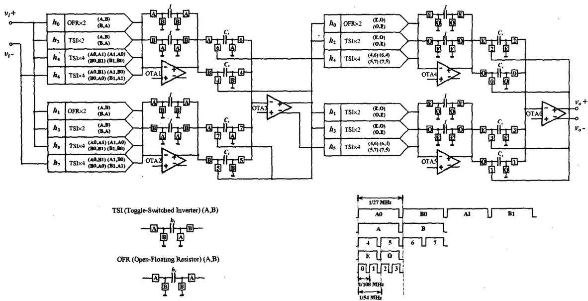
Fig.2 Simplified schematics and clock phases of 2-Stage SC FIR video anti-imaging filter
