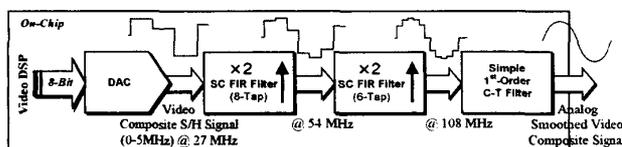
Fig.1 Low-cost analog interface for digital video by 2-Stage SC FIR anti-imaging filter
