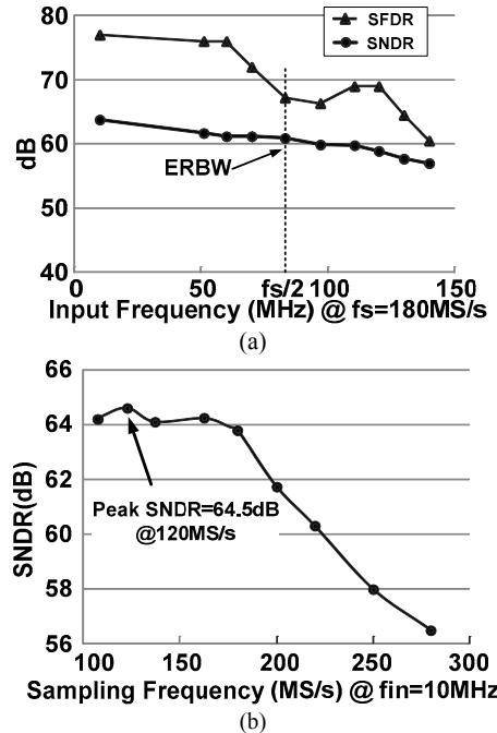
Fig. 9. Measured dynamic performances. (a) SNDR/SFDR vs. input. (b) SNDR vs. clock frequency.
