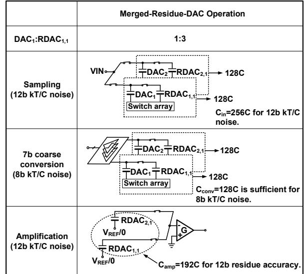
Fig. 3. The 1<sup>st</sup>-stage DAC operation with the noise performance in different phases.
