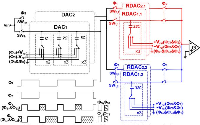
Fig. 2. Implementation of the 1<sup>st</sup>-stage DAC (single-ended).
