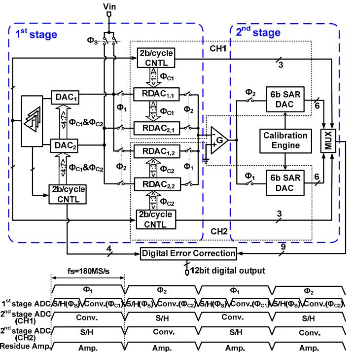
Fig. 1. PI Pipelined-SAR ADC architecture and timing diagram.
