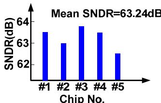
Fig. 7. Measured SNDR of 5 chips @ fin=10MHz, fs=180MS/s.
