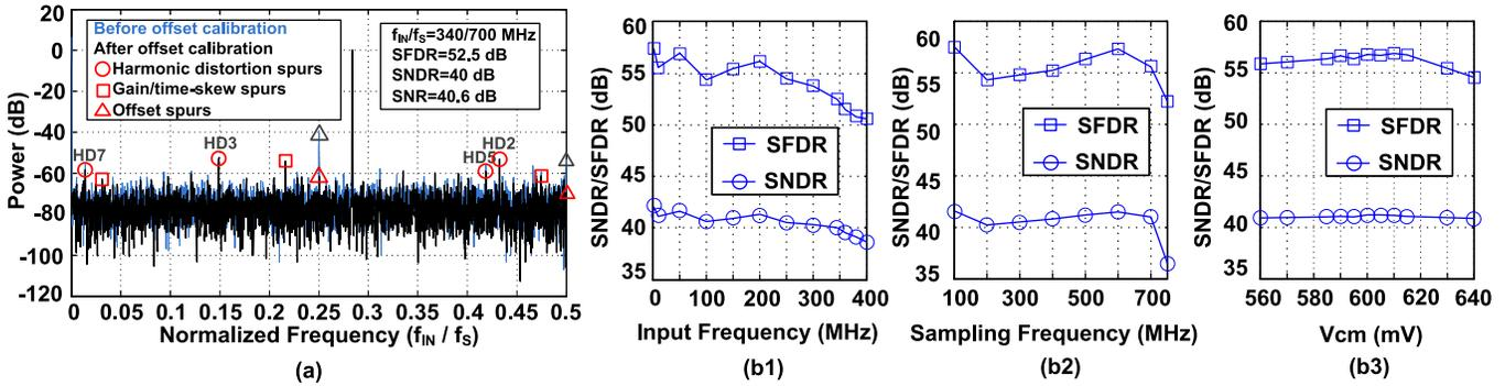
Fig. 6. (a) Measured 8192-point power spectrum at near-Nyquist input with  $f_s = 700$  MHz (decimated by 125). Measured dynamic performance SNDR and SFDR versus (b1)  $f_{IN}$  at  $f_s = 700$  MHz, (b2)  $f_s$  at  $f_{IN} = 10$  MHz, and (b3)  $V_{cm}$  reference voltage at  $f_{IN} = 10$  MHz and  $f_s = 700$  MHz.
